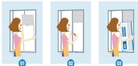
Tighten the bolts to secure the installation kit. Mount the installation kit on the window. Install the air conditioner in the installation kit
